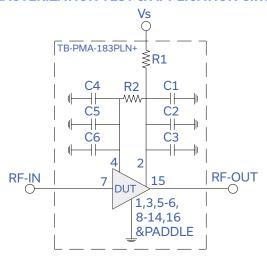
Fig 1. Application and Characterization Circuit
