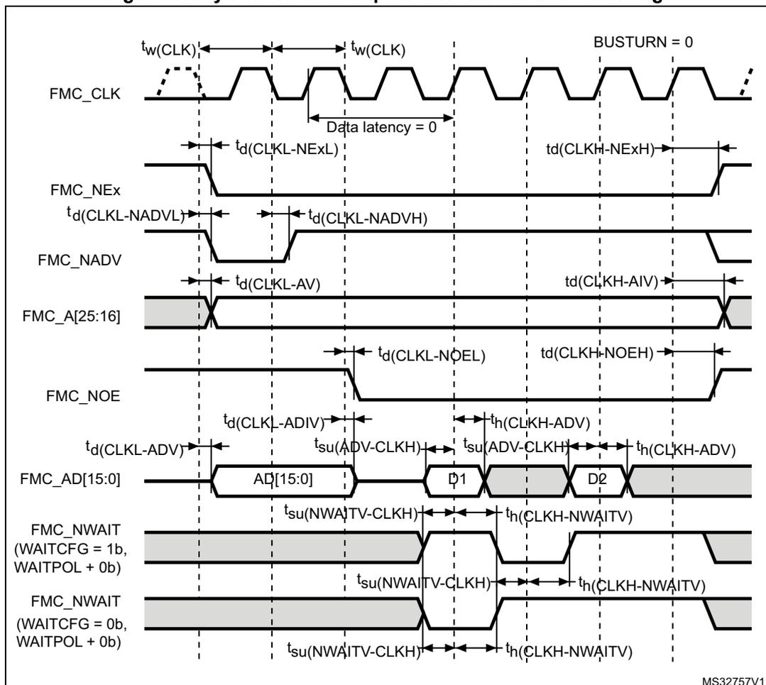
**Table 102. Synchronous multiplexed NOR/PSRAM read timings<sup>(1)(2)(3)</sup>**
