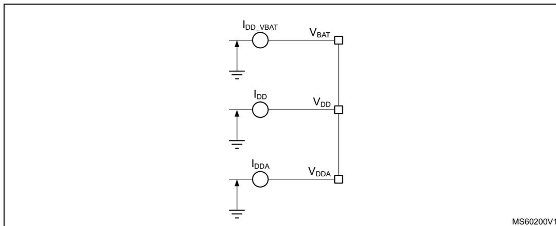
The  $I_{DD\_ALL}$  parameters given in [Table 21](#) to [Table 25](#) represent the total MCU consumption including the current supplying  $V_{DD}$ ,  $V_{DDA}$  and  $V_{BAT}$ .
