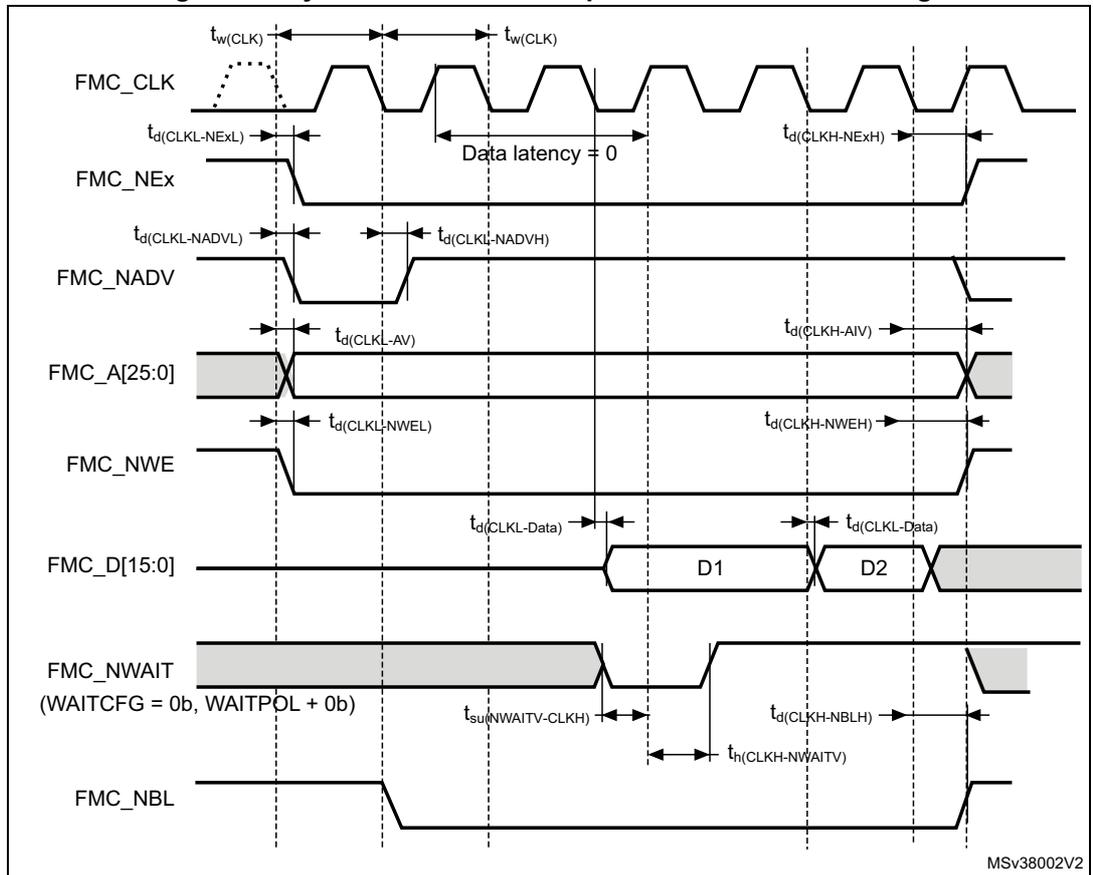
Table 105. Synchronous non-multiplexed PSRAM write timings<sup>(1)(2)(3)</sup>
