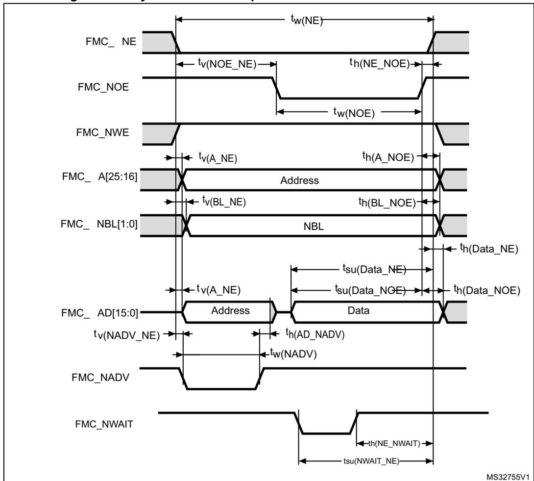
**Table 98. Asynchronous multiplexed PSRAM/NOR read timings<sup>(1)(2)</sup>**
