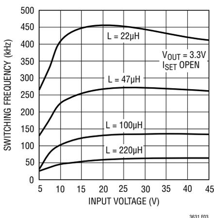
Figure 3. Switching Frequency for  $V_{OUT} = 3.3V$
