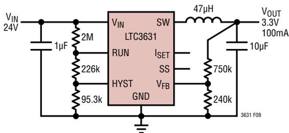
Figure 9. 24V to 3.3V, 100mA Regulator at 250kHz
