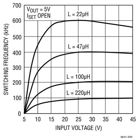
Figure 2. Switching Frequency for  $V_{OUT} = 5V$
