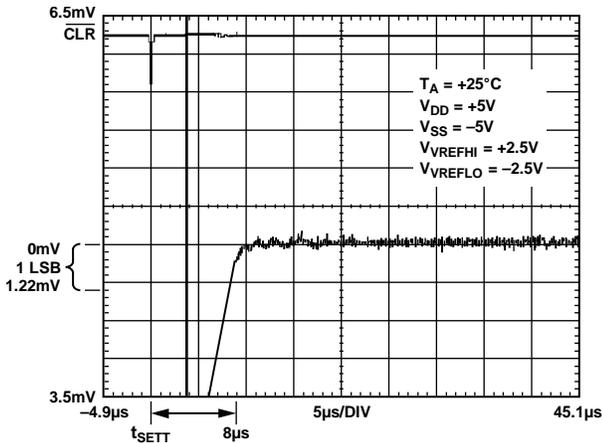
Figure 20. Negative Settling Time ( $\pm 5$  V)
