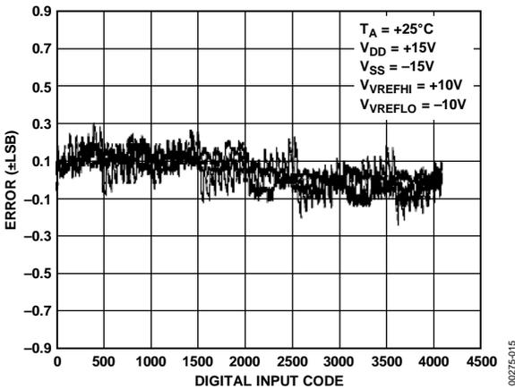
Figure 14. Channel-to-Channel Matching
