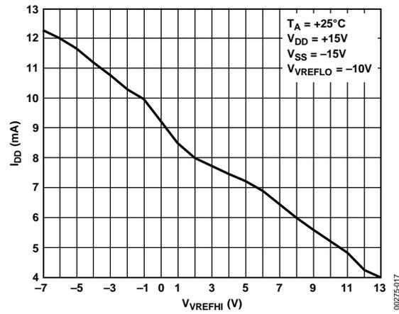
Figure 16.  $I_{DD}$  vs.  $V_{REFHI}$  All DACs High
