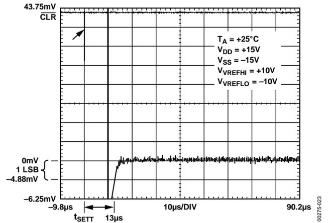
Figure 22. Negative Settling Time ( $\pm 15$  V)
