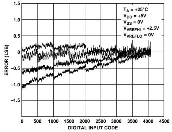
Figure 15. Channel-to-Channel Matching
