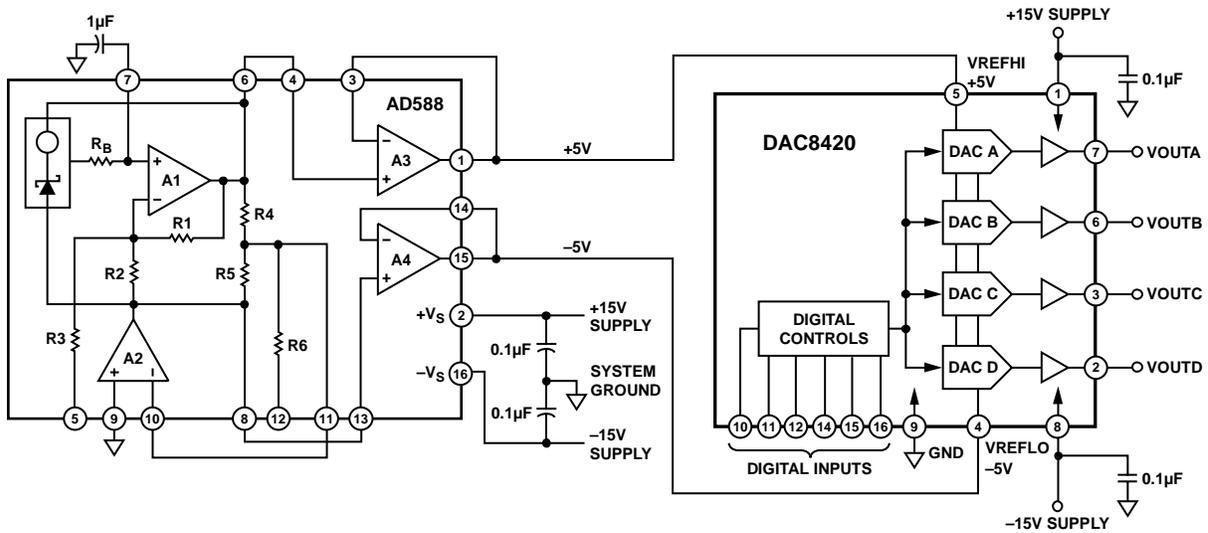
Figure 33. ±10 V Bipolar Reference Configuration Using the AD588
