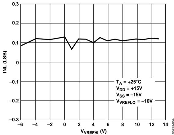
Figure 8. INL vs.  $V_{REFHI}$  ( $\pm 15$  V)
