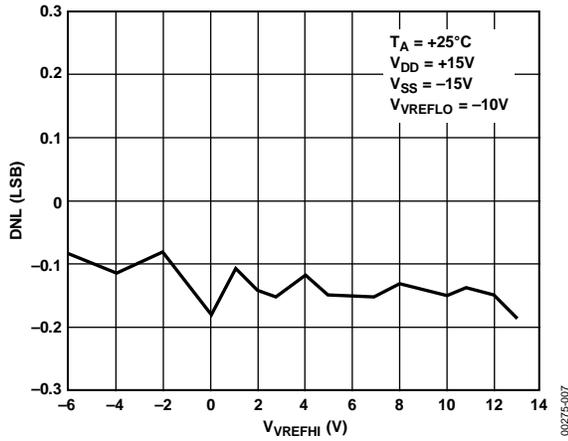
Figure 6. DNL vs.  $V_{REFHI}$  ( $\pm 15$  V)
