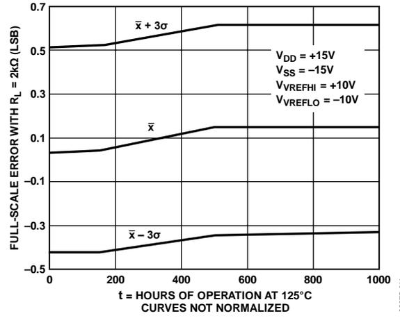
Figure 10. Full-Scale Error vs. Time Accelerated by Burn-In
