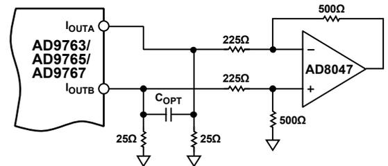
Figure 73. DC Differential Coupling Using an Op Amp
