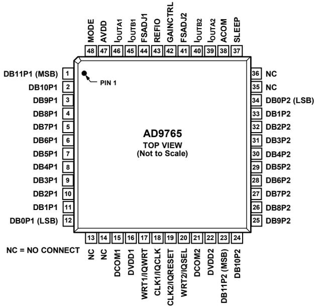
Figure 4. AD9765 Pin Configuration
