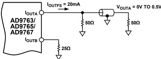
Figure 75. 0 V to 0.5 V Unbuffered Voltage Output
