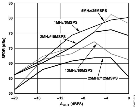
Figure 13. Single-Tone SFDR vs.  $A_{OUT}$  @  $f_{OUT} = f_{CLK}/5$
