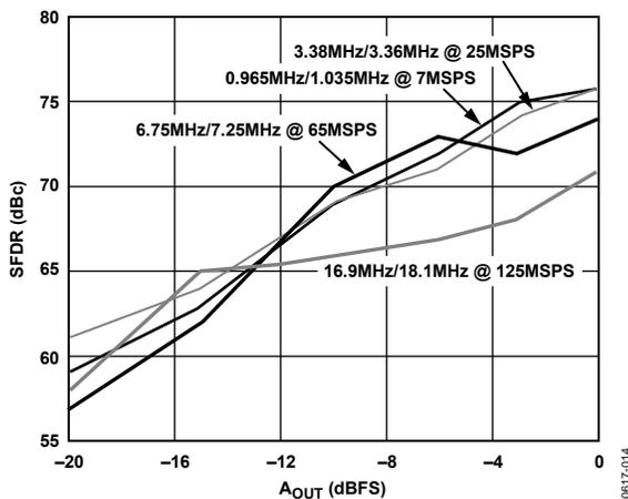
Figure 14. Dual-Tone SFDR vs.  $A_{OUT}$  @  $f_{OUT} = f_{CLK}/7$
