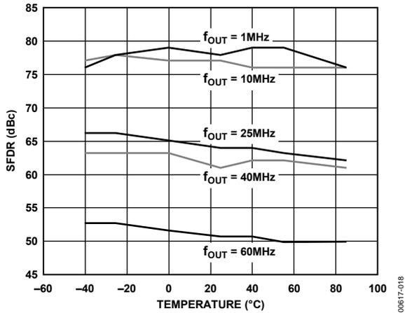
Figure 18. SFDR vs. Temperature @  $f_{CLK} = 125 \text{ MSPS}$ , 0 dBFS
