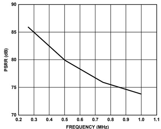
Figure 77. AVDD Power Supply Rejection Ratio vs. Frequency
