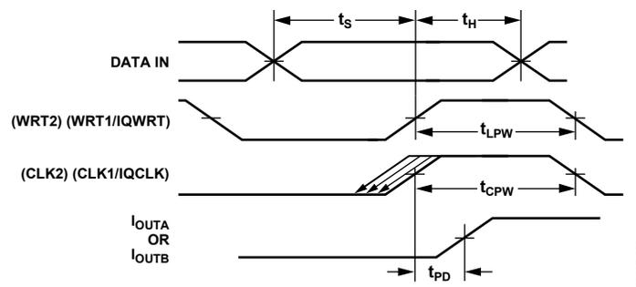
Figure 2. Timing Diagram for Dual and Interleaved Modes
