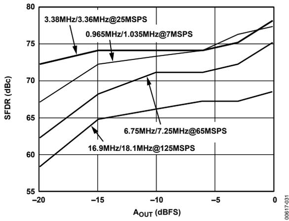
Figure 31. Dual-Tone SFDR vs.  $A_{OUT}$  @  $f_{OUT} = f_{CLK}/7$
