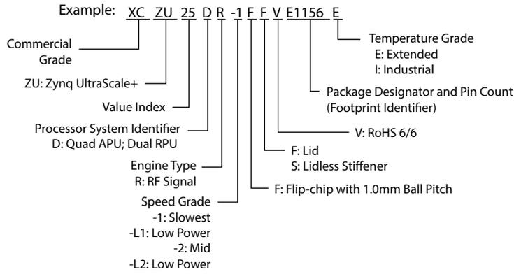
1) -L1 and -L2 are the ordering codes for the low power -1L and -2L speed grades, respectively.
